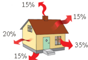
Figure 3.1 – Typical heat losses of a house (Municipality of Sundsvall 2009)
