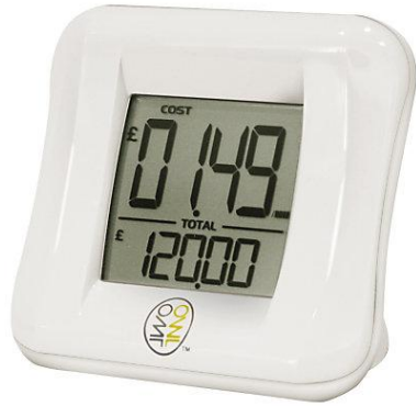
Figure 5.2 – The OWL Micro display, providing real-time feedback on cost (John Lewis Partnership 2009)
