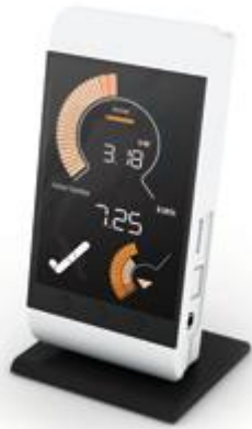
Figure 5.3 – The Solo display by Green Energy Options, equipped with historic feedback (Green Energy Options 2009)
